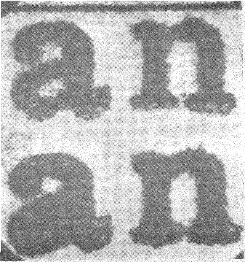
Fig. 7. Photomicrograph of letters purportedly typed on same date. Note difference in amount of ink in typewriter ribbon, indicated by degree of blackness and the fact that open portions of bottom "a" is filled with ink. (See text.)
